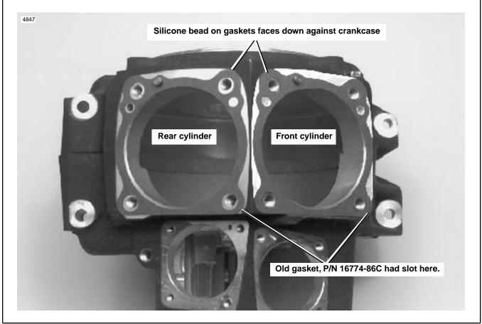
Figure 3. New Gaskets Installed On Crankcase
