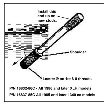
Figure 2. New Cylinder Studs.
